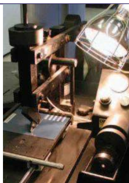
SCRATCH ADHESION TEST
